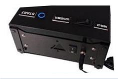
Turn on the power switch ("I" position). The **status light** turns blue in a few seconds.
