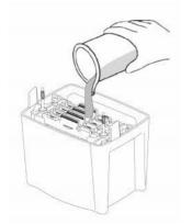
6. Put the cold cooling unit in the tank and fill up the tank by buffer.
