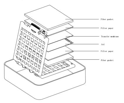
Note: In order to achieve the best blot result, it is key to remove the air bubble by glass bar stirring.
