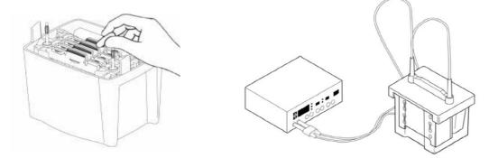
9. Disassemble the sandwich when the electrophoresis ends, take out the membrane and continue the next step. Use the neutral detergent to rinse the electrophoresis tank, blot clip, macroporous sponge, and then again use the ion-removing water to rinse.
