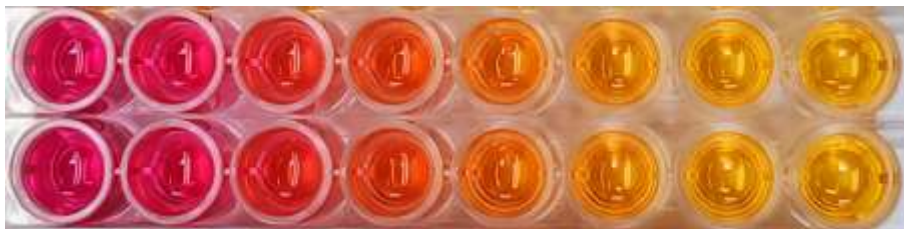
Figure 1: Example Zinc Standard Curve (100 \mu\text{M} to 0 \mu\text{M} ) in a 96-Well Microtiter Plate (0.78 and 0.39 \mu\text{M} points omitted).
